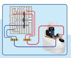
The advantages of flow reversal when descaling and chemical cleaning
