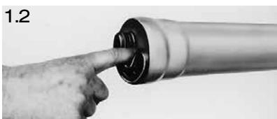
1.2 Push in sealing element at the top with fingers so that it fills the seal chamber until the collar of the sealing element is positioned evenly on the socket rim. Brush sealing element inside and slip-in pipe outside thoroughly with **LORO-X lubricant**.
